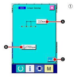
Display the linear ordinary sewing setting screen. Select and execute LINEAR ORDINARY SEWING (function code 023) → 023 in the code list screen, and the linear ordinary sewing setting screen is displayed.
