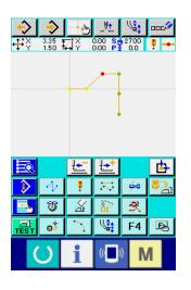
In case of the relative point move, the whole pattern data after the moved point moves while holding the previous relation.
