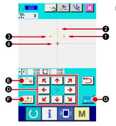
Press MOVE key  $\underbrace{\leftarrow} & \underbrace{\rightarrow} & \textcircled{O}$  in the coordinate input screen, and the needle position moves in the specified direction. When DECIDING POINT button  $\underbrace{\leftarrow} & \textcircled{O}$  is pressed, the shape point of the linear ordinary sewing is inputted. When PASSING POINT button
