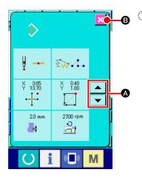
Display the contents of pattern display screen. Press PATTERN CONTENTS DISPLAY button in the standard screen, and the contents of pattern display screen is displayed. Contents to be displayed can be changed over with UP/DOWN SCROLL buttons and screen et urns
