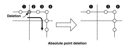
As the result of deleting the point, be careful that the distance of change does not exceed the maximum stitch length of the sewing machine.
