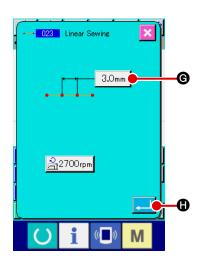
Select the linear ordinary sewing (function code 023) in the function code list screen, and press ENTER button .
