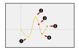
Point (B) can be moved by moving both point of rear (2) and point of front (3) to the same coordinates.
