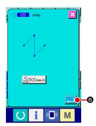
Press ENTER button **[]** in the jump feed setting screen to display the jump feed position specifying screen.
