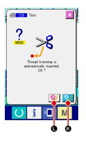
In the case where the thread trimming command does not exist in the termination of pattern and before jump feed, the automatic thread trimming insertion confirmation screen is displayed after pressing SEWING PREPARATION button
