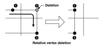
In case of the relative vertex deletion, the whole pattern data after the deleted point moves while holding the relation before deletion.
