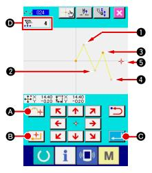
Input the breakpoint in the spline ordinary sewing. Select the spline ordinary sewing (function code 024) in the code list screen, and perform the coordinate input of the spline ordinary sewing. Input points 1, 2 and 4 with PASSING POINT button A and point 3 and point 5 with
