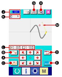
The figure on the right-hand side is the position specifying screen which is displayed when specifying the position at the setting of function. The selected function code is displayed at **①**.
