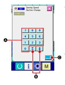
① Display the sewing speed section change setting screen. Press SEWING SPEED SECTION CHANGE button in the standard screen or select and execute SEWING SPEED SECTION CHANGE (function code 061) SECTION CHANGE (function code 061) in the code list screen, the sewing speed section change setting screen is displayed.
