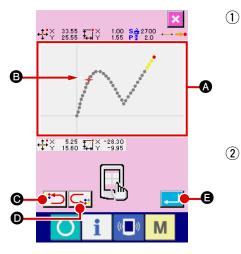
Display the needle entry/shape points instructions screen. When COORDINATE INSTRUTIONS button is pressed in the screen specifying needle entry/shape points such as the standard screen, the shape point specifying screen, etc., the needle entry/shape points instructions screen is displayed.
