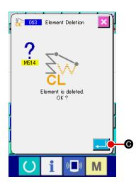
Press ELEMENT DELETION button 👔 🕒 in the standard screen, and press ENTER button 🛋 👁 in the confirmation screen.
