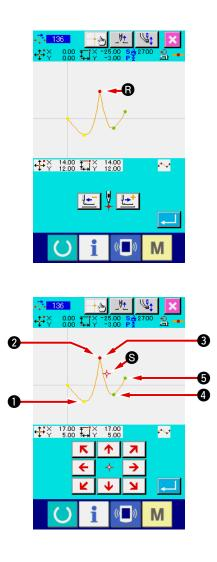
When you desire to move point (a) to point (b), the result will be changed by selecting either shape point of rear (2) or front (3).
