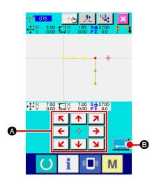
The point is added after the specified needle entry point. The pattern data after the added point does not move. Point adding can be added to not only the pattern data created with the input of point sewing, but also the data inputted with any function such as linear sewing or the like.
