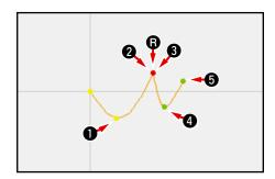
When performing the shape point deletion of either point of rear 2 or point of front 3, the breakpoint becomes the normal passing point and the continuous spline sewing is formed.
