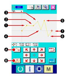
Input the breakpoint in the ordinary sewing. For the ordinary sewing, the point to be inputted is determined according to the kind of element immediately before the point where DECIDING POINT button Select ORDINARY SEWING (function 022) Select ORDINARY SEWING (function 022) and input points (), (2), (5) and (7) with DECIDING POINT button (3) and points (3), (4) and (5) with PASSING POINT button
