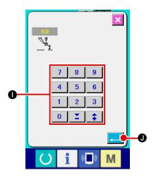
(d) When PRESSER HEIGHT SETTING button is pressed, the intermediate presser reference value setting screen is displayed.
